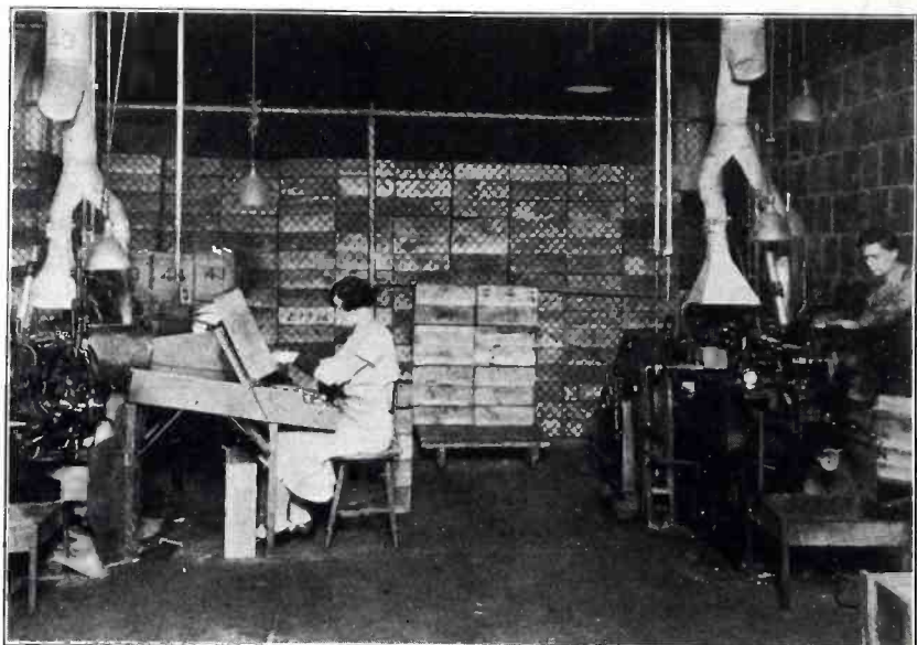
Above is an automatic machine which turns out zinc cans with soldered seams
