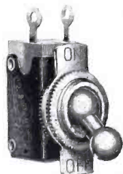
POWER TOGGLE SWITCH —For power sets, Eliminators, Chargers. Compact, rugged. Quick make and break action. Und. Lab. Insp. 3A-125v=1A-250v. (Actual Size)
