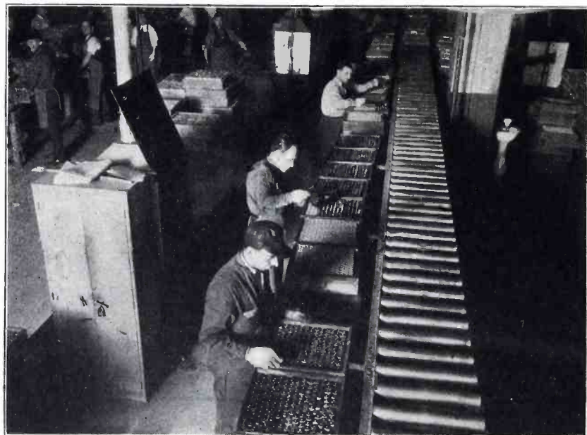
At the left the workmen are sealing the cells by pouring melted wax into the tops
